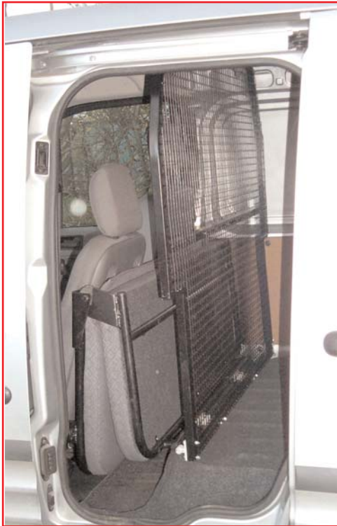
Seat folded up with mesh bulkhead moved forward still leaving 85% of the vans carrying capacity
