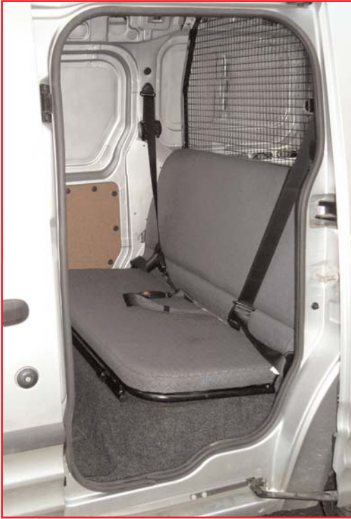
Seat in place with optional moveable bulkhead, 2 lap and diagonal seat belts and one lap belt and carpet kit
