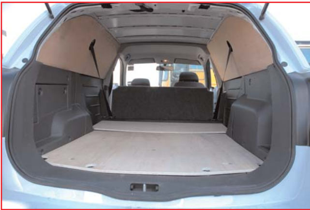
Seat kit folded down showing the woodlined floor which is supplied with the seat kit. It also shows the above plastic woodline kit that we supply as an extra
