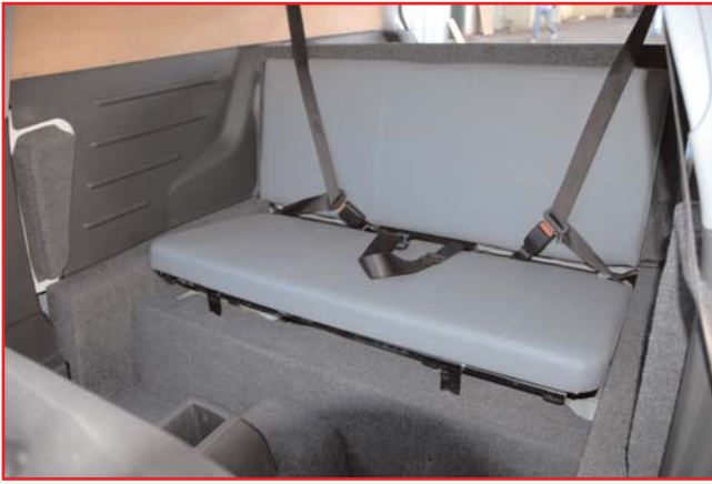
Seat from front showing 2 x lap and diagonal seat belts and a lap belt in the middle
